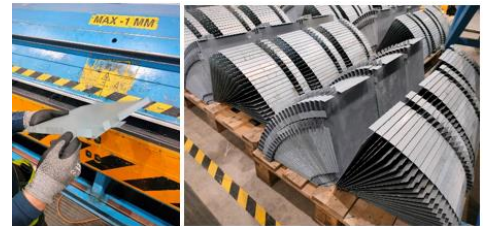
Bending the tiles.
