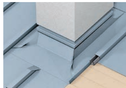
Abb. 52: Connection to chimney with front flashing (version with continuous soldered cleat)
