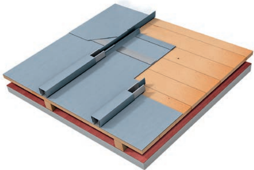
Fig. 33: Cross seam with soldered continuous cleat
