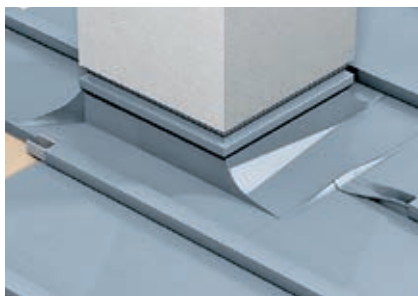
Abb. 51: Connection to chimney with wedge-shape back gutter and roll cap adapter in double standing seam technique
