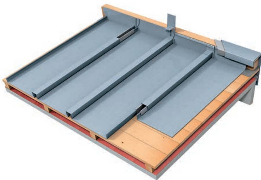
Fig. 28: Mono pitch ridge with ridge termination cap and ridge flashing
