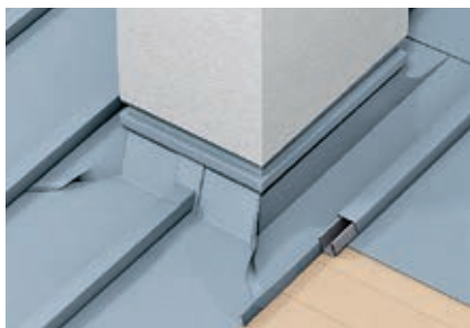
Abb. 50: Connection to chimney at front with ridge upstand and ridge cap
