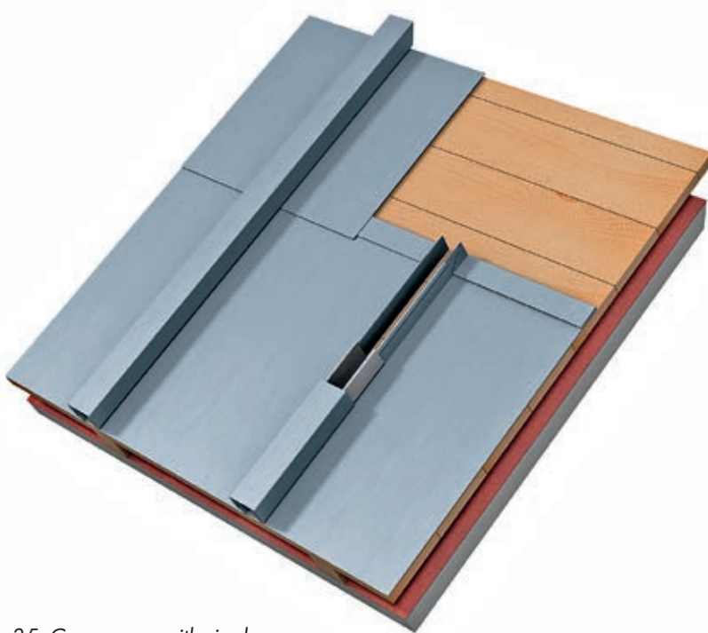
Fig. 35: Cross seam with single seam
