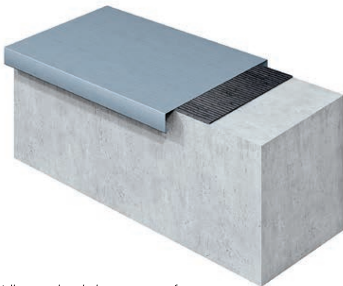
Fig. 5: Wall coping bonded over entire surface
