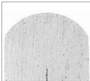
Fig. 3: Metallographic cross section of a flexural test piece after a 180° fold, without an intermediate layer, parallel to rolling direction
