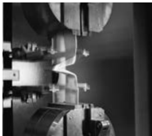
Fig. 2: Tensile seam test in the RHEIN-ZINK-Quality Control Dept.
