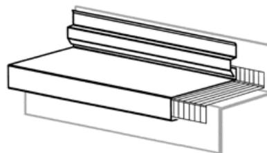
Detail of join, cornice coping with cover flashing and UDS-Connector
