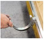
Lock each bracket into place by twisting it 90 degrees clockwise.
