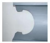
Cut out the second half including 2 strips at the side each approx. 50 x 20 mm
